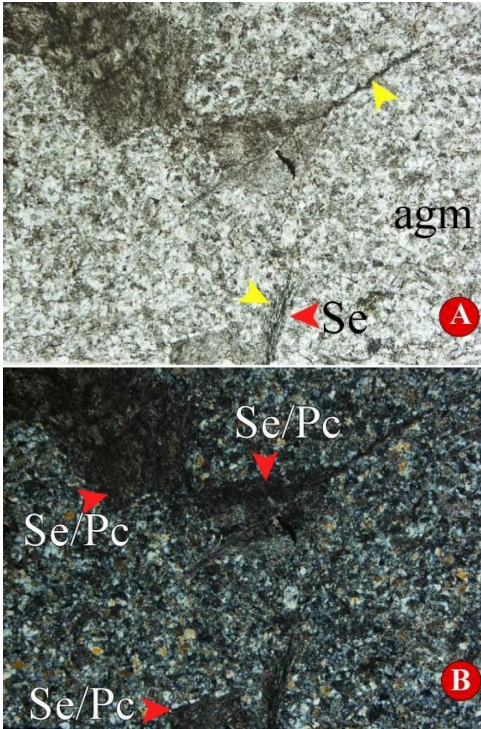
Plate 6. Photomicrographs, A -plane light, B -crossed nicols, show the sericite-filled discontinuous micro fractures (yellow arrows) filled with sericite in the altered groundmass (agm) comprised of
